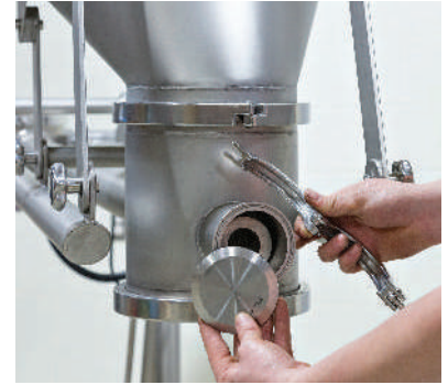
Quick disassembly - fast reassembly - tool-less cleaning
