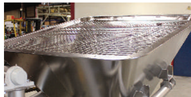
Bolted-in safety grate
