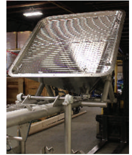
Hopper corners are rounded for easy cleaning
